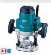
Continuous rating input 1,650W Collet Capacity 12.7mm Plunge Capacity 0-60 mm Plunge Capacity Base dia. 160x148mm No Load Speed (r/min) 22,000 Dimensions (L x W x H) 284x148x300mm Net weight 5.5kg Power supply cord 2.0m
